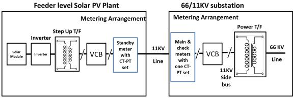
(Indicative Diagram: Metering Arrangement Lay out)
