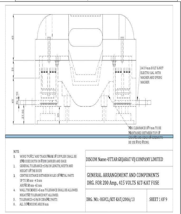
**Drawing of SMC Fuse Box for 200 Amp Kit Kat Fuse**
