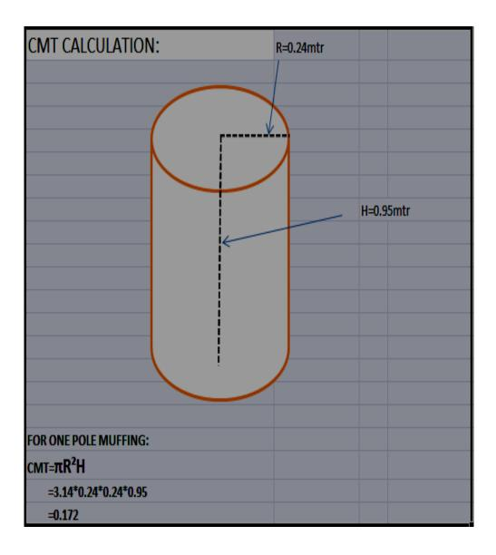
As per drawing, the standard size of Pole muffing is 0.172 CMT & rates are to be quoted accordingly. However, actual size may vary as per site situation & quantity will be considered accordingly.
